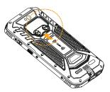
. Turn the screw, open the SD card waterproof cover
