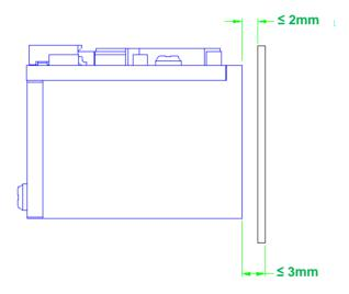
If the window is required to be in a tilted position, the distance requirements above should be met and tilt angle should ensure no reflections back into the lens.
