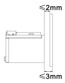
If the window is required to be in a tilted position, the above distance requirements should be met and tilt angle should ensure no reflections back into the lens.
